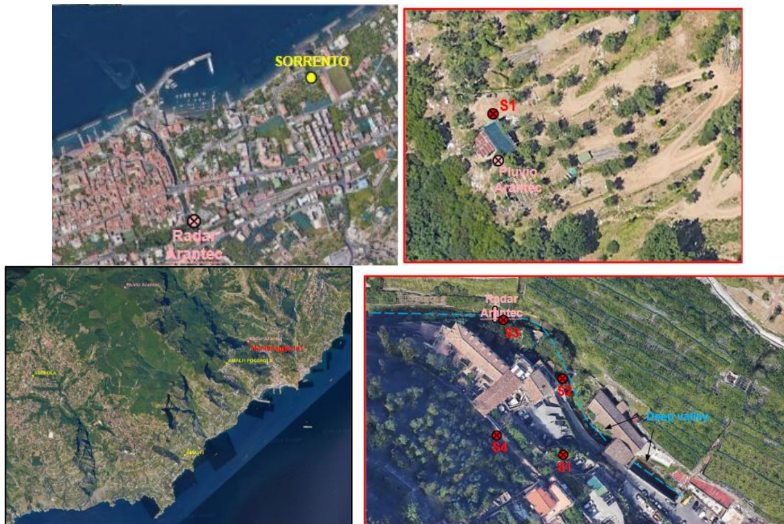
Figure 4: Location of sensors in Sorrento and Amalfi in situ monitoring stations; (first row) left: the location of radar for measurements of water discharge in Sorrento; right: pluviometer and investigated soil profiles in terms of volumetric water content. (second row) left: location of additional rain gauge identified as “Pluvio Arantec”; right: S1,S2, S4 identify soil volumetric water content investigated profiles while S3 identifies the location for radar measuring water discharge; center.
