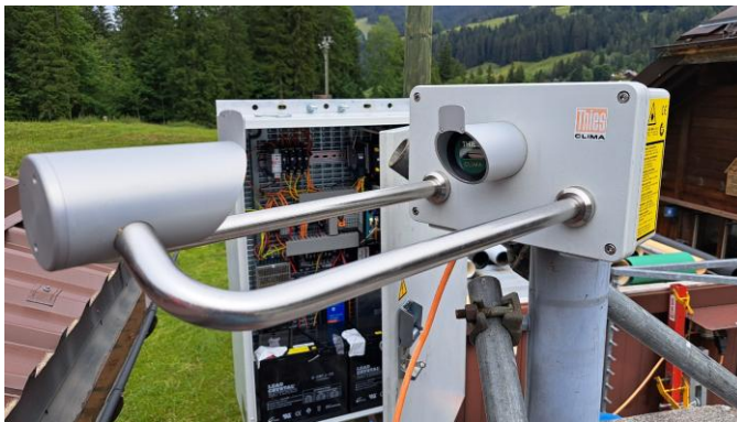
Figure 11: (left) a view of Thies disdrometer installed in Zug; (right) kinetic energy and momentum as returned by the disdrometer for a convective event occurred in the area on July, 31 2024
