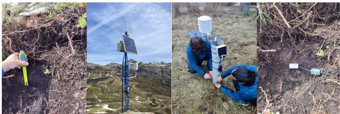
Figure 3: Installation of new monitoring stations within the DEM2; ( from left to right: excavation for sensor installation, installed weather station, researchers engaged in sensor installation, volumetric water content sensors installed horizontally on the excavation face.
