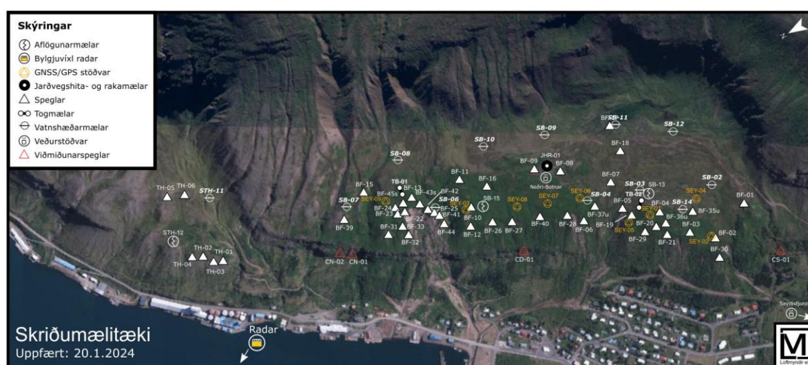
Figure 6: Monitoring stations in Seyðisfjörður; it represents a clear example of diffuse monitoring including, among the others, extensimeters, sensors for soil volumetric water content and temperature, discharge levels, weather stations (DEM6)
